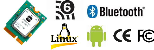
SPB437 WiFi6 2x2 concurrent dual Wi-Fi module
